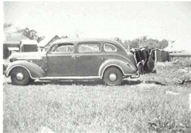
Above: Dodge car at Appin with charcoal-burner fitted to rear. Ca. 1943. Image courtesy of Campbelltown and Airds Historical Society, NSW. http://server2.webfrogstudios.com.au/welcome-to-our-website.html
